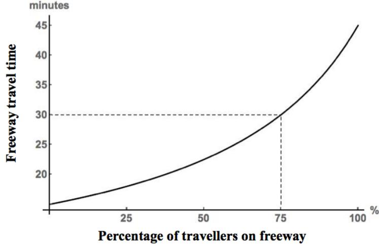
**Figure 1. Freeway travel time increases non-linearly with freeway traffic [see Equation (1)].**
